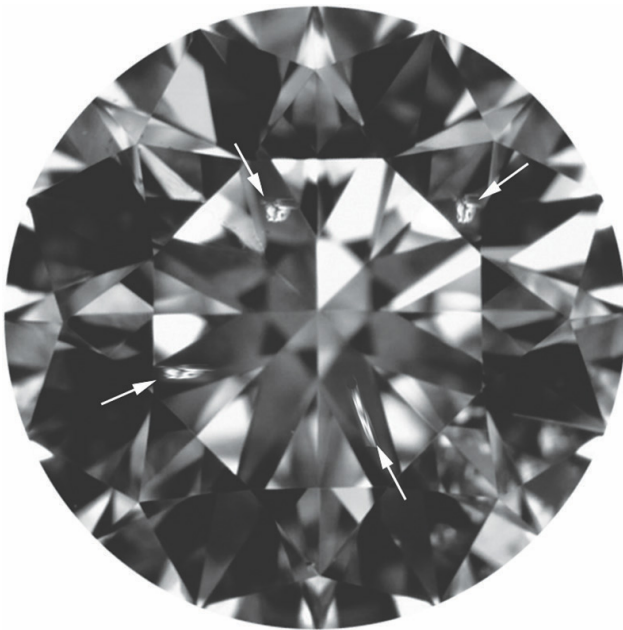
Figure 2: This 1.11 ct diamond (6.66–6.63 x 4.11 mm) contains four SI-1 size inclusions that have different dimensions, but the same area and contrast, and thus, similar visibility. Each has an area determined to be approximately .035mm 2
