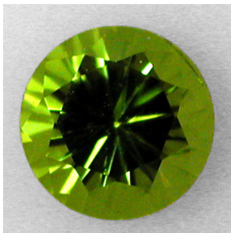
Figure 16. Nailhead round brilliant peridot cut with 45° pavilion main angle.
