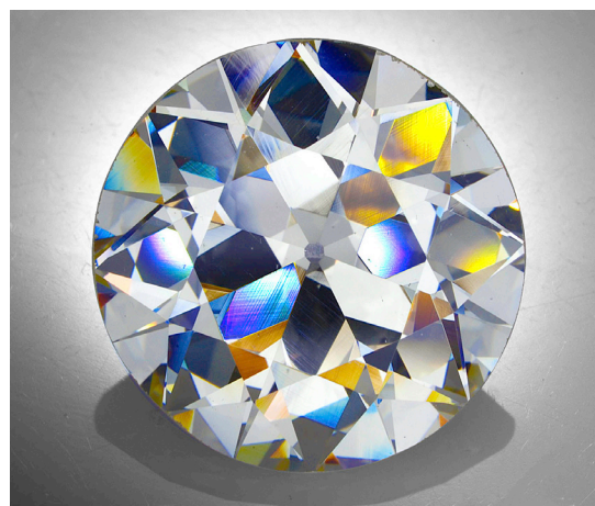
Figure 5. Early Ideal cut with its 16 dominant virtual facet reflections from the 8 large pavilion main facets.
