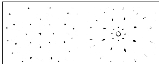
Figure 6 (L). Reflection pattern from the crown of a red garnet recorded on photographic paper in the plate P by the reflectograph in the Figure 4 configuration. Figure 7 (R). Reflection pattern of a deep blue sapphire, brilliantly ground (very regular) recorded on photographic paper in the plate P by the reflectograph also in the Figure 4 configuration.
