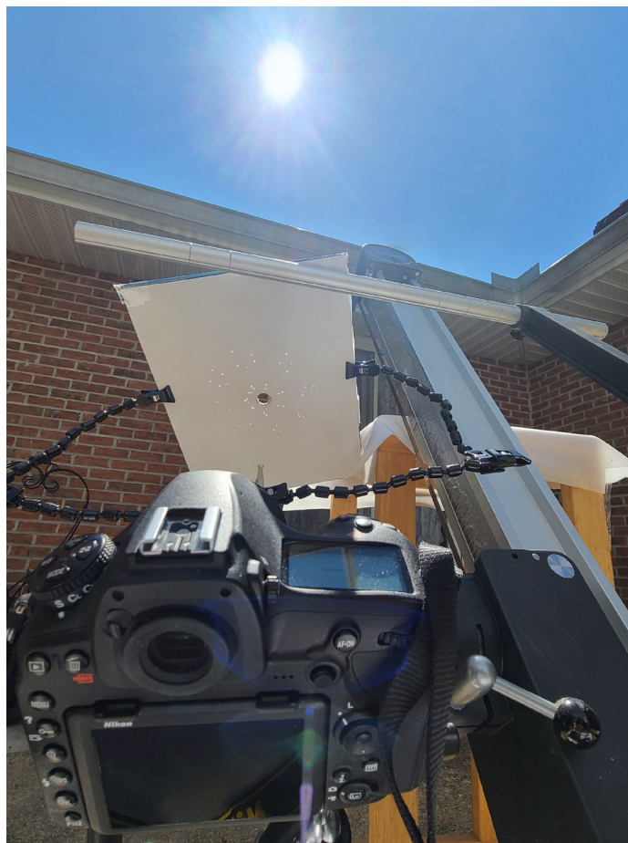
Figure 1. Setup to generate and photograph a diamond's Spectral Reflection Pattern utilizing a beam of light from the sun
