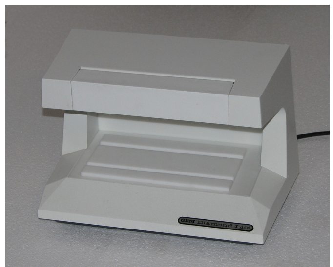
4. GIA DiamondLite containing two Verilux F6T5 fluorescent tubes.
