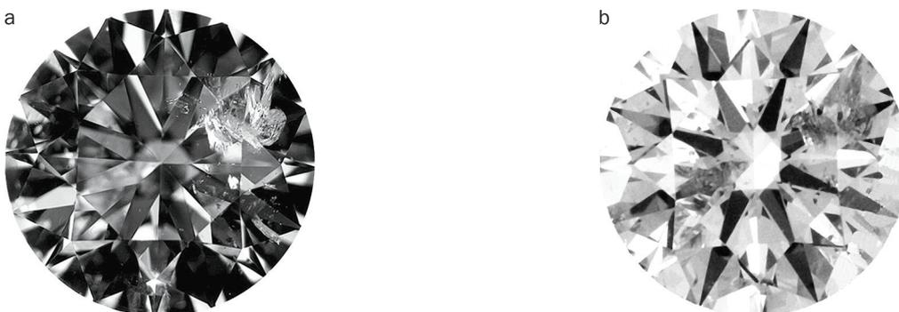
Figure 21: This 0.35 ct  $I_2$ -graded diamond ( $4.55\text{--}4.54 \times 2.78$  mm) contains a large  $I_1$ -size fracture that is best seen with darkfield illumination (a). Viewed with overhead lighting (b), a reflection of the fracture causes a doubling of its apparent area, which combined with the relatively small size of the diamond leads to a solid  $I_2$  clarity grade.
