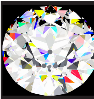
Figure 24. 41°, 35°, 45% American Cut, Tilted Away 20°
