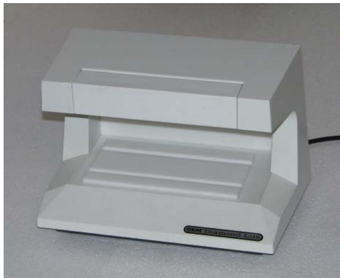
Figure 8: GIA DiamondLite containing two Verilux F6T5 fluorescent tubes.
