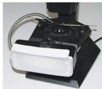
Figure 10: Microscope light fitted with white diffuser and Lexan UV filter.
